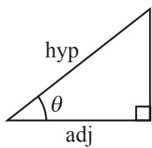
$$\begin{aligned}\text{adj} &= \text{hyp} \times \cos \theta \\ \text{opp} &= \text{hyp} \times \sin \theta \\ \text{opp} &= \text{adj} \times \tan \theta\end{aligned}$$
